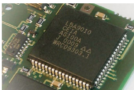
Proprietary Engineering consisting of a powerful analytical engine designed exclusively by CEIA specifically for metal detection
