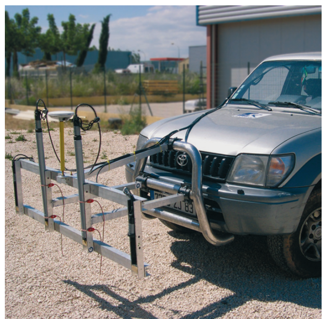
Vehicle-mounted multi-channel system
