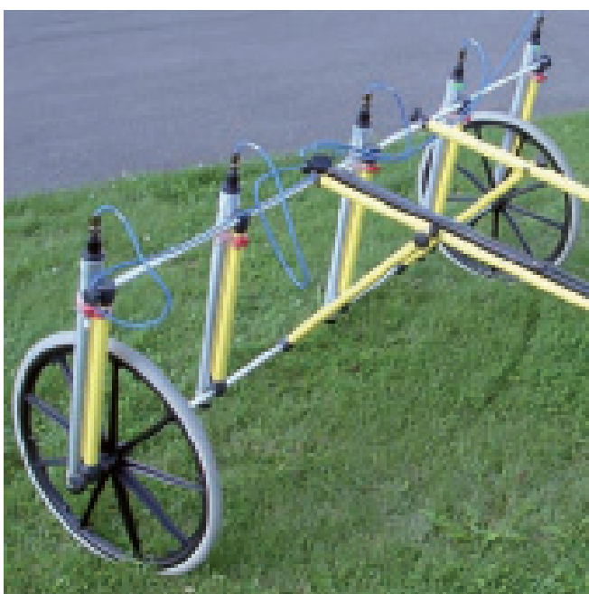
5-channel system MAGNEX® 120 LW
