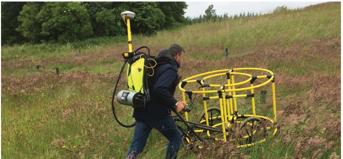
Figure 1. Example use of the UPEX® 745 DF with GPS in difficult terrain
