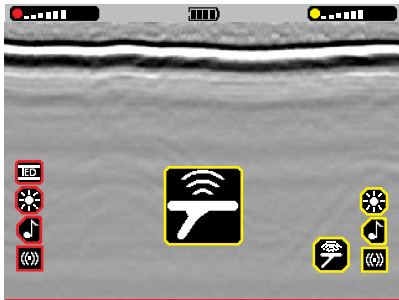
Bad Skyshot: horizontal bands are present in the GPR Imagery when the detector is still raised.
