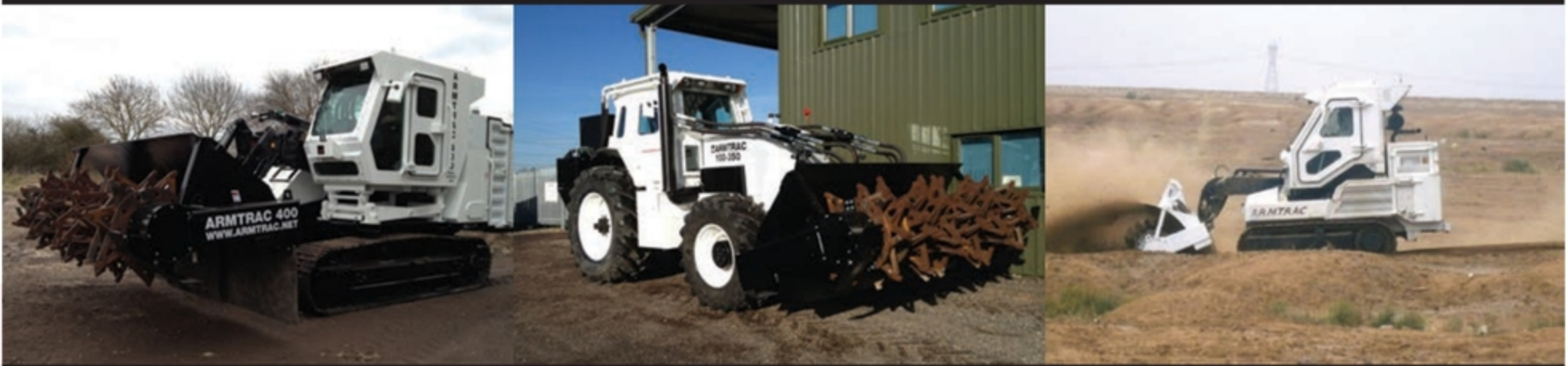
Armtrac 400 - the largest and most powerful of Armtrac's humanitarian demining equipment
