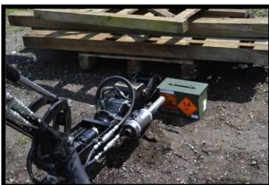
Disrupter on the Excavator Arm
