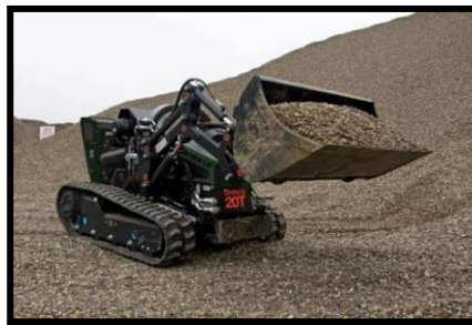
Front loader bucket with 300kg of stone
