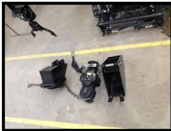
Strimmer, Clam shell and bucket
