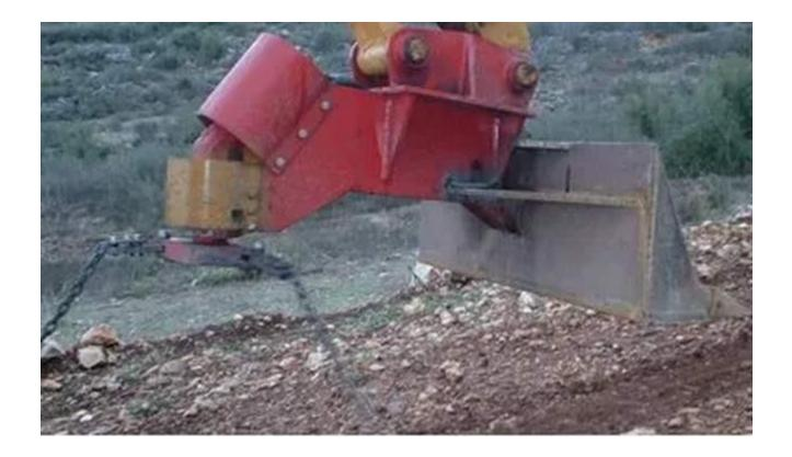
**The Armtrac Strimmer** is designed as an aid in ground UXO clearance, specifically for difficult to reach areas where none of Armtrac's other machines are able to reach. As with all Armtrac products, the **Armtrac Strimmer** is armoured to withstand Anti-tank mines.
