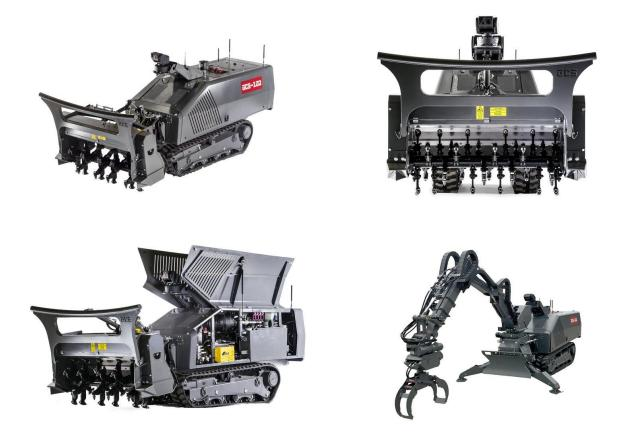
The GCS-100 is the smallest of our two available platforms and outperforms any similar product on the market. It's a versatile, compact, remote-controlled platform suited for Technical Survey, Anti-Personnel minefields, C-IED, Runway and Route Clearance in ultra-rugged, hard-to-access urban environments.
